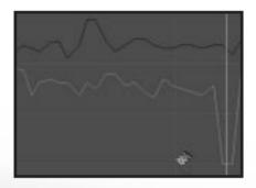
A transfer of vertical load of this type is an advantage for a car that understeers: because of this transfer, there will be a load shift to the front axle which will increase its efficiency making it possible to increase cornering speed. On the other hand, if there's too much transfer of vertical load a car behaving neutrally, or even oversteering, the removal of load from the rear axle may put the car into a spin.
